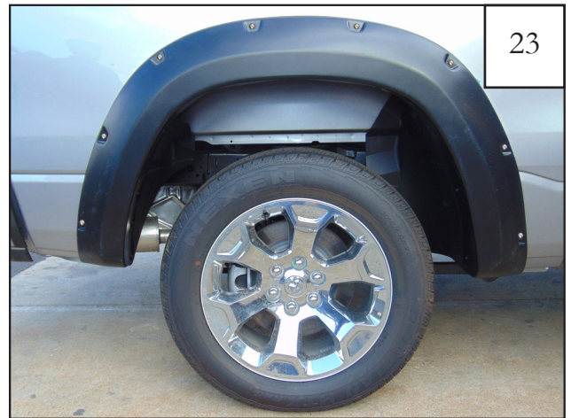
Completed rear flare installation.
